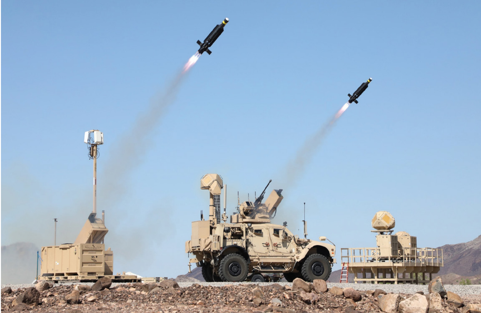
Two variants of the Coyote 2C drone interceptor are fired during testing at the Yuma Proving Ground, Arizona, in 2021. The kinetic interceptors provide the U.S. Army with a flexible short-range counter-unmanned aircraft system capability. (Photo courtesy of the U.S. Army)
