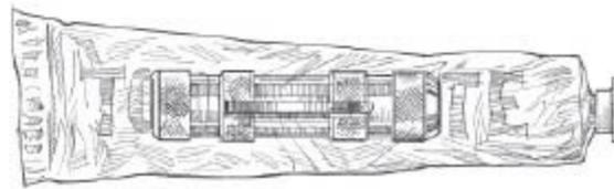
A toothpaste tube used as concealment for the CIA STINGER, a small .22-caliber single-shot firing device.
