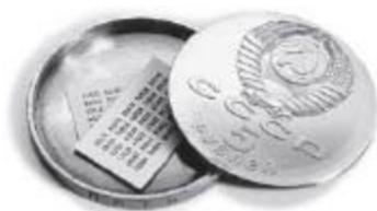
Russian spy coin machined to create a cavity for concealing soft film and ciphers. The coin opened by inserting a small tool (or needle) into the loop of the numeral 9 in the date, 1991, on the bottom face of the coin.
