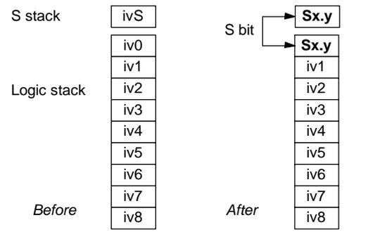
Figure 6-31 Effect of LSCR on the Logic Stack
