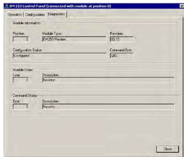
Figure 9-19 Diagnostics Tab of the EM 253 Control Panel
