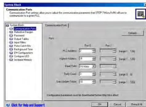
Figure 7-4 Configuring the S7-200 CPU
