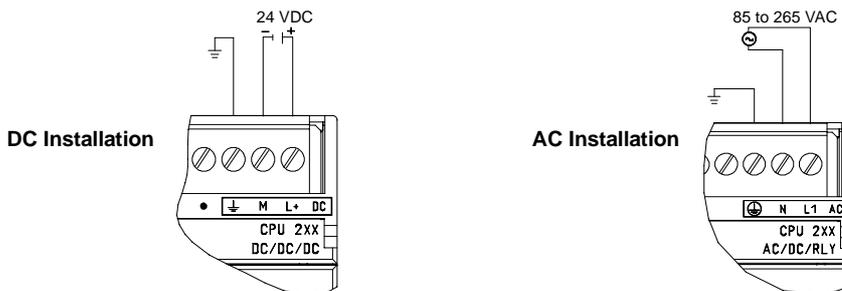
Figure 2-1 Connecting Power to the S7-200 CPU
