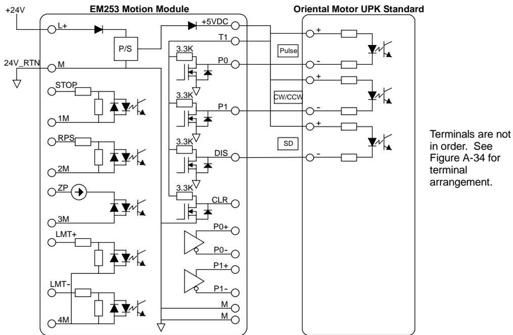
Figure A-38 Connecting an EM 253 Position Module to an Oriental Motor UPK Standard
