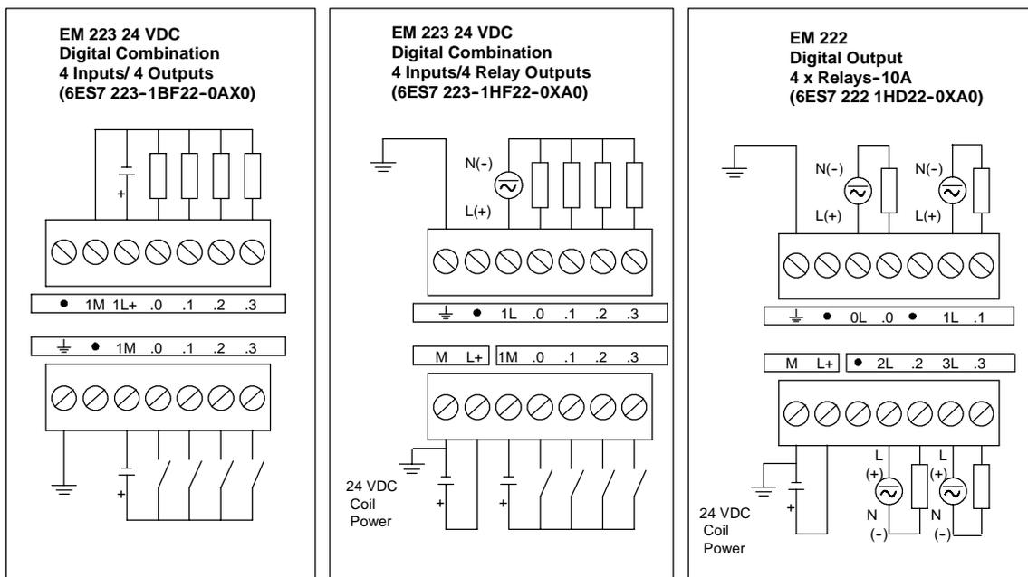
Figure A-9 Wiring Diagrams for EM 222 and EM 223 Expansion Modules
