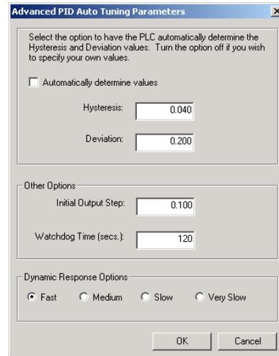
Figure 15-3 Advanced Parameters
