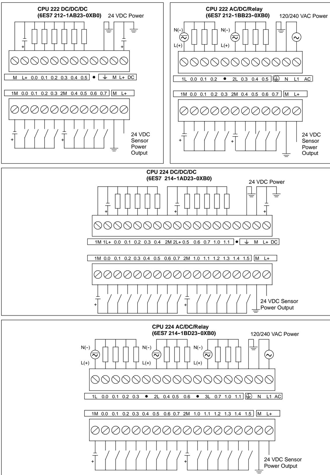
Figure A-4 CPU 222 and CPU 224 Wiring Diagrams
