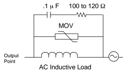
Figure 3-4 Suppression Circuit for an AC Load
