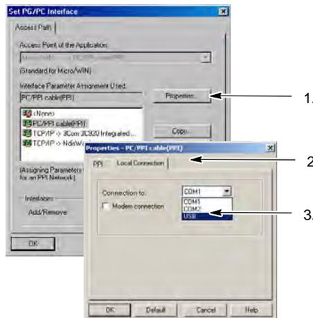
Figure 7-2 PPI Multi-Master Cable Selection
