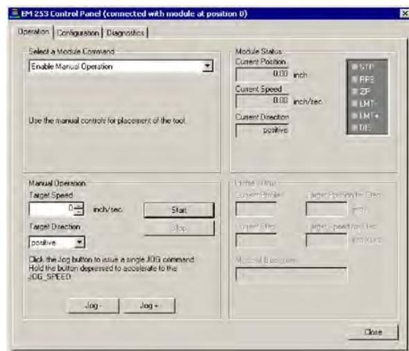
Figure 9-17 Operation Tab of the EM 253 Control Panel
