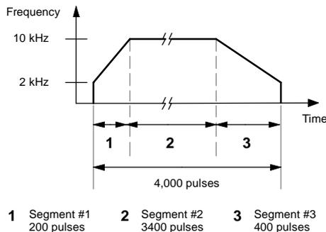
Figure 6-30 Frequency/Time Diagram
