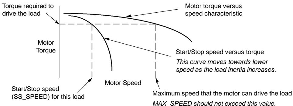
Figure 9-4 Typical Torque-Speed Curve for a Motor
