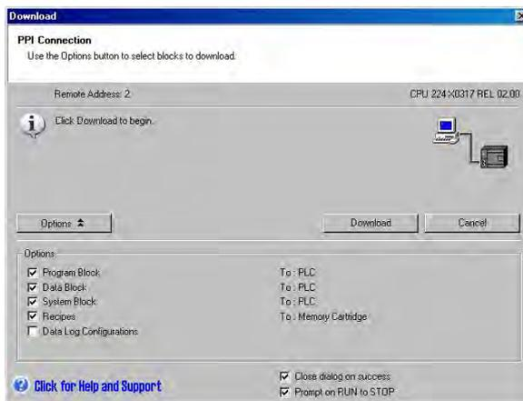
Figure 13-7 Downloading a Project with Recipe Configuration
