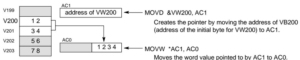
Figure 4-12 Creating and Using a Pointer
