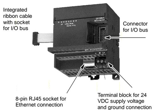
Figure A-40 Connecting the (CP 243-1) Ethernet Module
