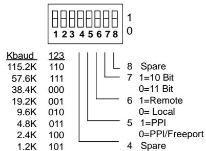
Figure 7-29 Settings for the RS-232/PPI Multi-Master Cable
