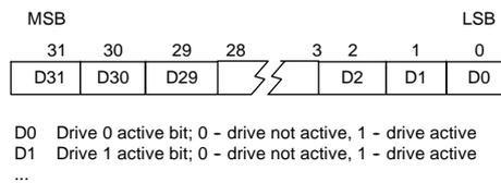
Figure 11-2 Format for the Active Drive Parameter
