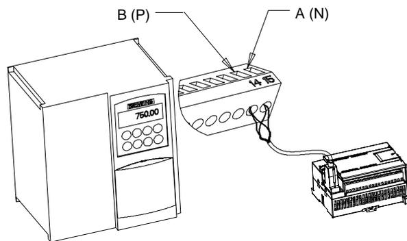
Figure 11-6 Connecting to the MM420 Terminal Block
