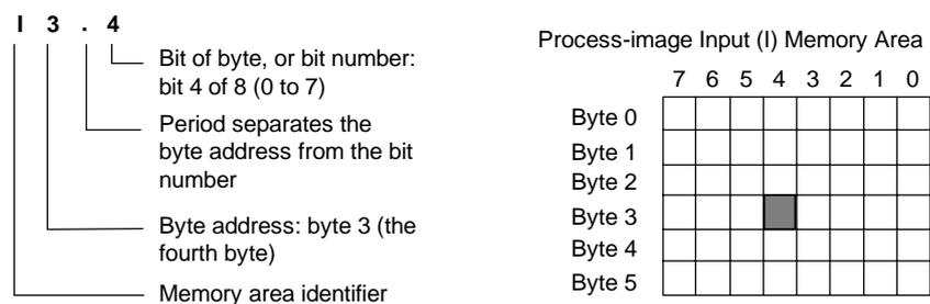
Figure 4-4 Byte.Bit Addressing
