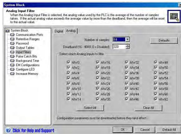
Figure 4-24 Analog Input Filter
