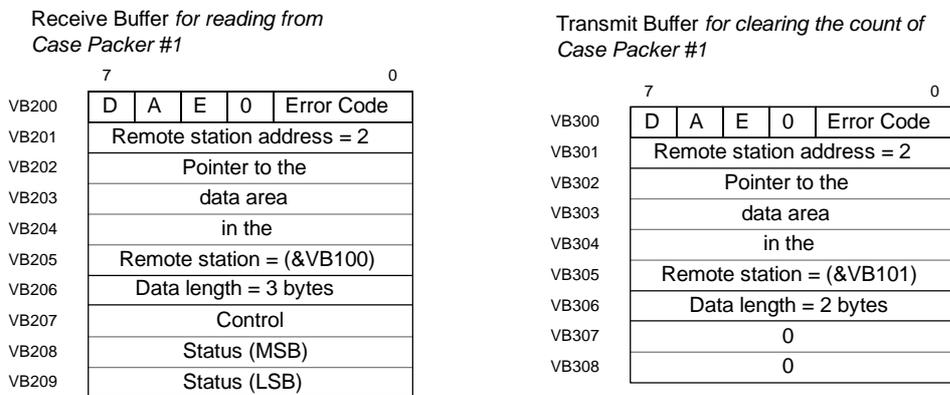
Figure 6-7 Sample TBL Data for the Network Read/Write Example
