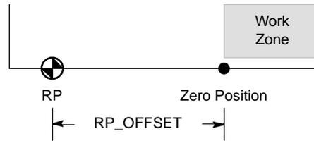
Figure 9-15 Relationship Between RP and Zero Position
