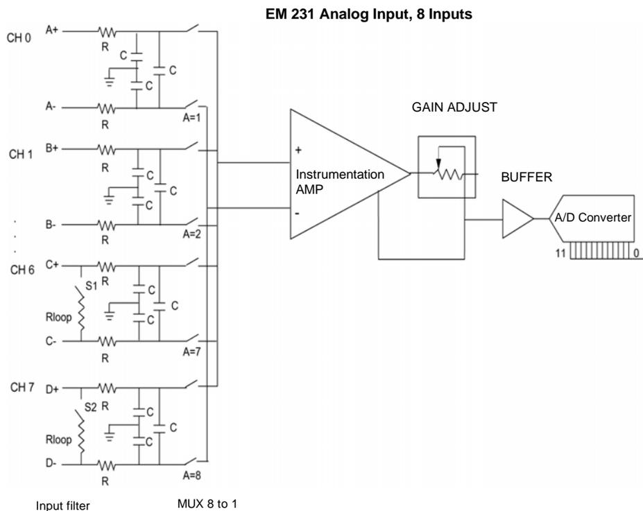
Figure A-18 Input Block Diagram for the EM231 Analog Input, 8 Inputs
