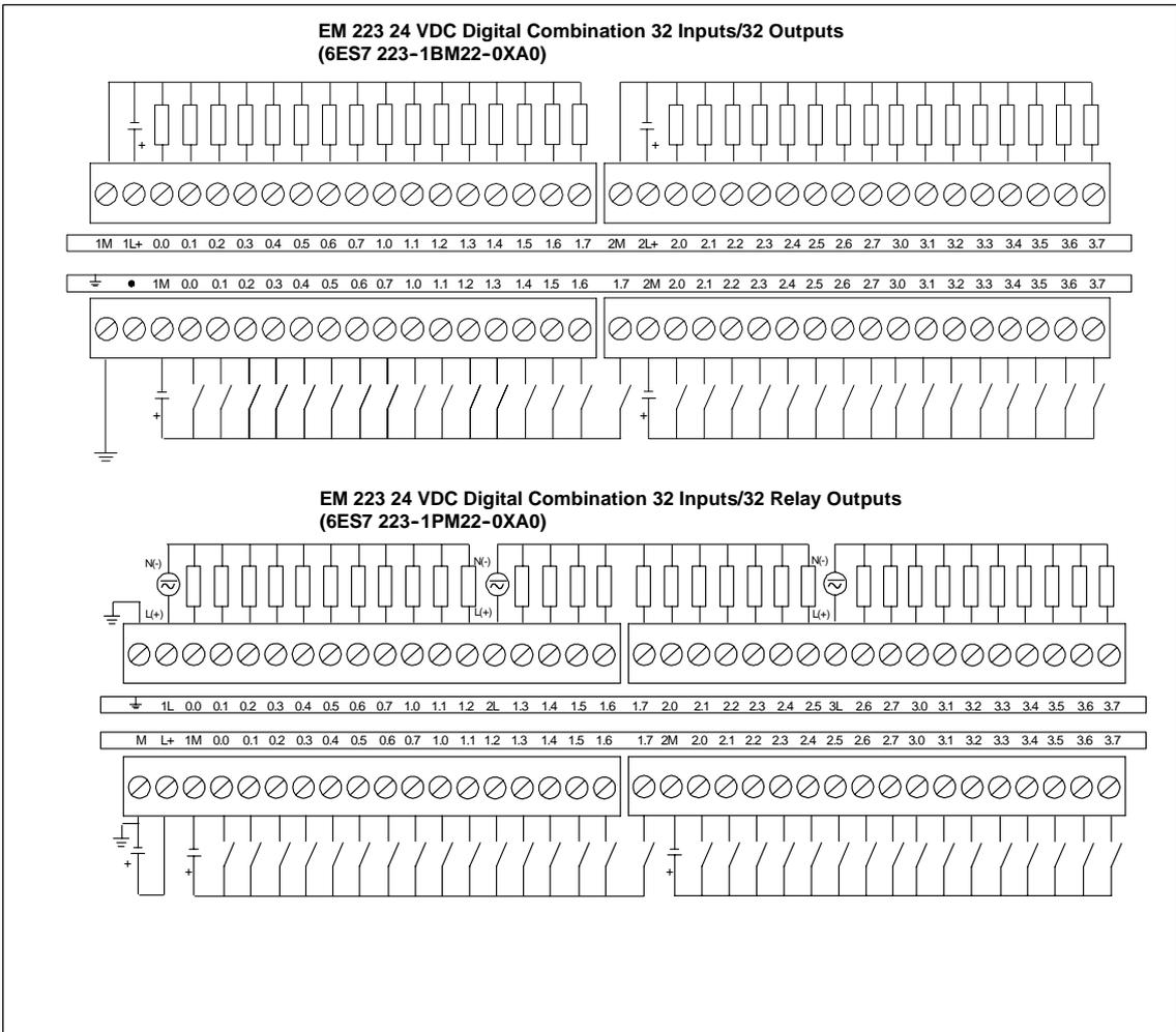
Figure A-12 Wiring Diagrams for EM 223 Expansion Modules
