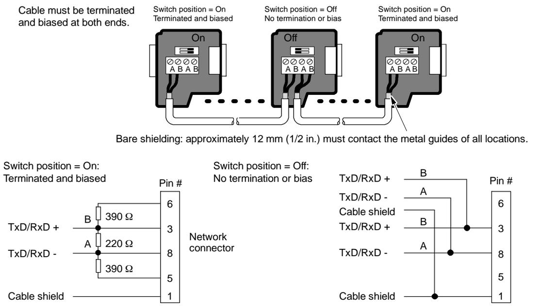
Figure 7-22 Bias and Termination of the Network Cable
