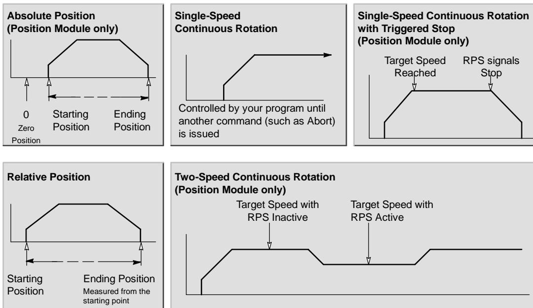
Figure 9-6 Mode Selections for the Position Module
