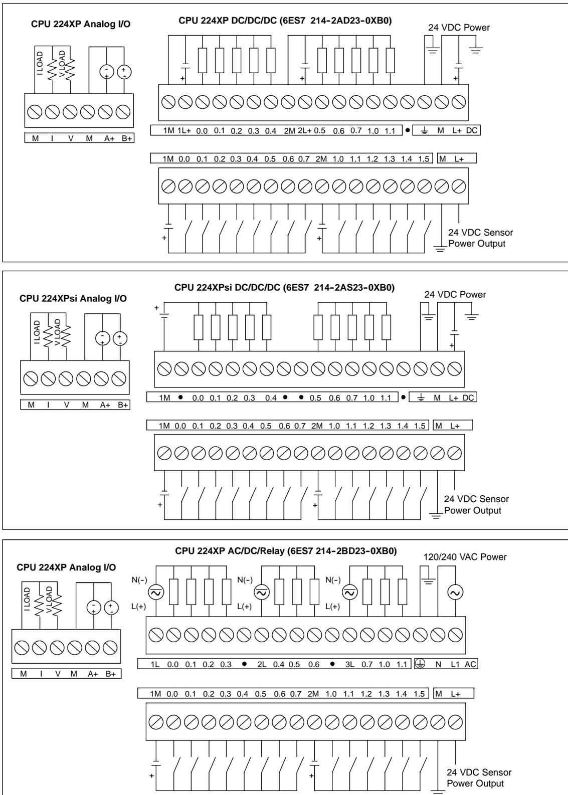
Figure A-5 CPU 224XP Wiring Diagrams
