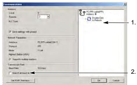
Figure 7-6 Searching for CPUs on a Network
