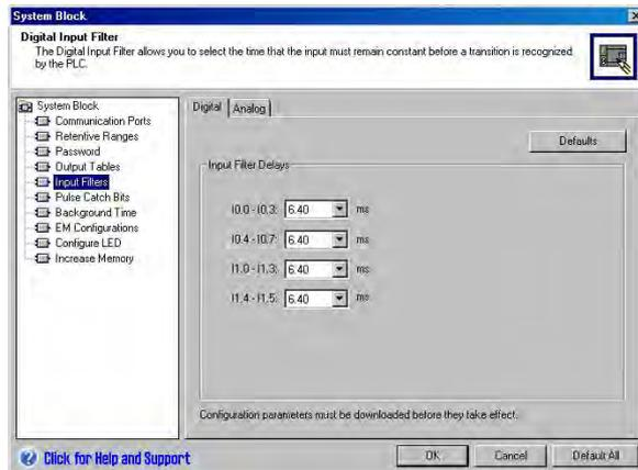
Figure 4-23 Digital Input Filter
