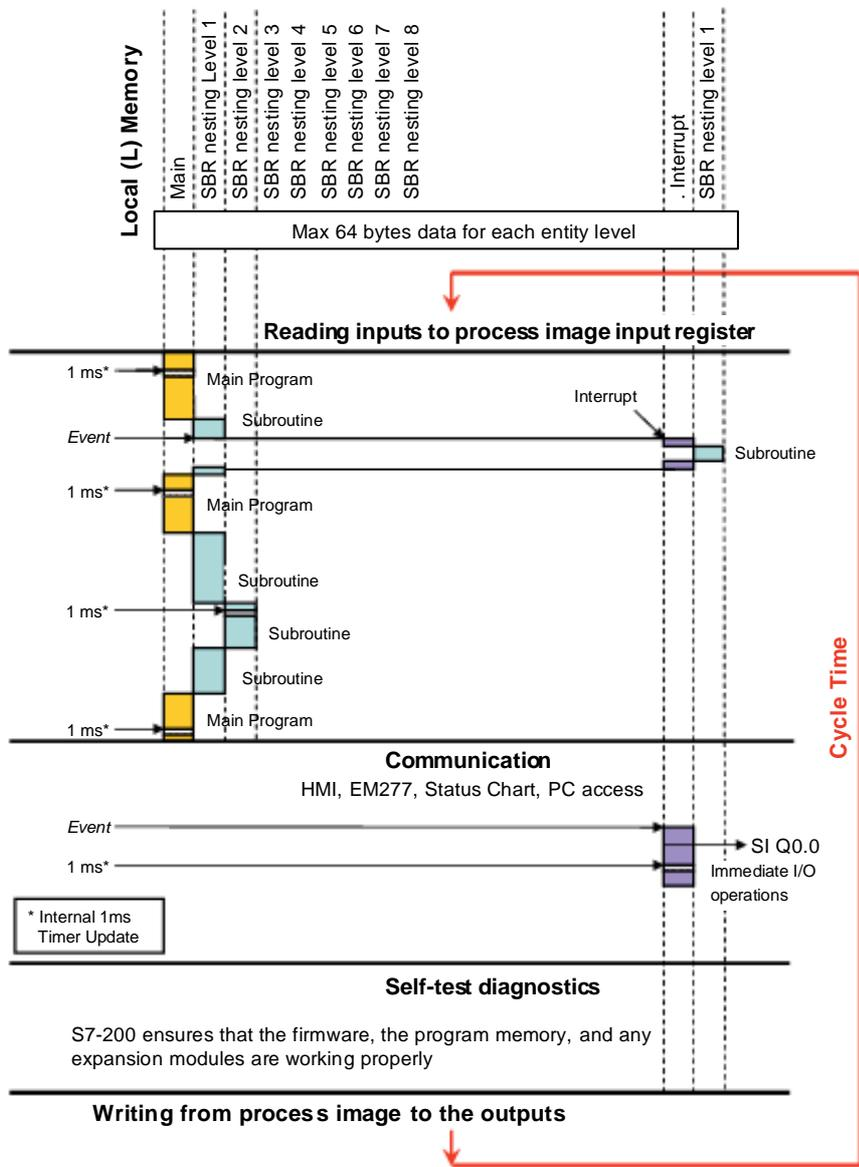
Figure 4-3 Typical Scan Flow
