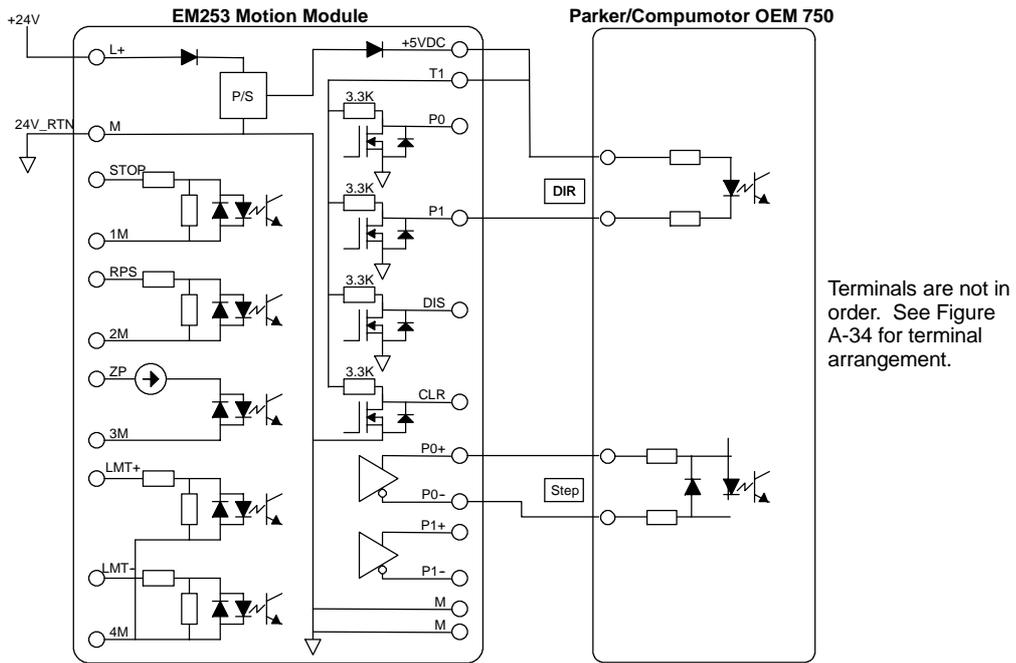
Figure A-39 Connecting an EM 253 Position Module to a Parker/Compumotor OEM 750
