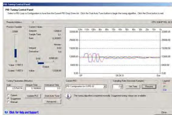
Figure 15-1 Auto-Tuning Sequence on a Direct Acting Loop
