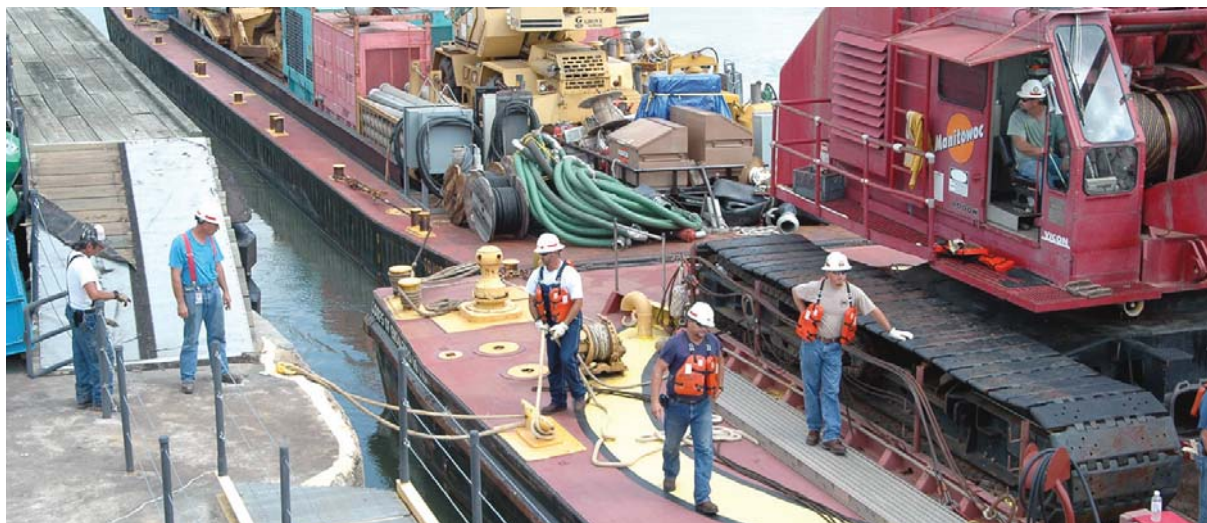
Two large loads of pumping equipment and their support crew from the Corps of Engineers Little Rock District pass through the Inner Harbor Navigation Canal Lock. The equipment was unloaded in New Orleans to help pump the water out of the lower Ninth Ward.
