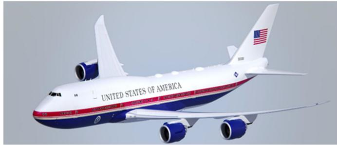
The modifications to the 747-8 aircraft will include an electrical power upgrade, dual auxiliary power units that are usable in flight, a mission communication system, an executive interior, military avionics, a self-defense system, autonomous enplaning and deplaning, and autonomous baggage loading.
