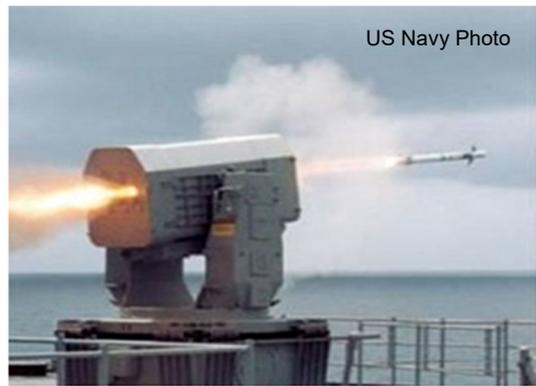
**Mission:** Provides high firepower close-in defense of combatant and auxiliary ships by utilizing a dual mode, passive radio frequency/infrared missile in a compact 21 missile launcher.
