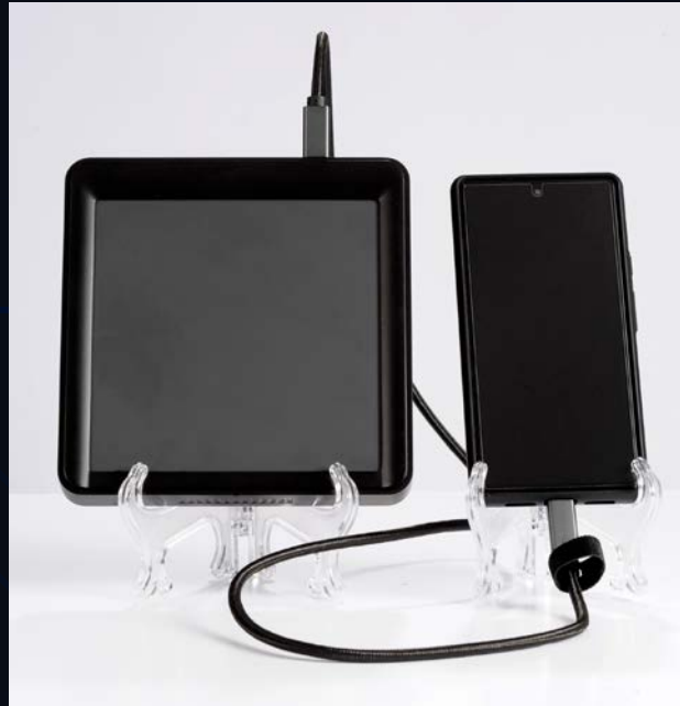
Above is an example of a Mobile Palm Print Capture Device attached to a Bureau issued cell phone.
